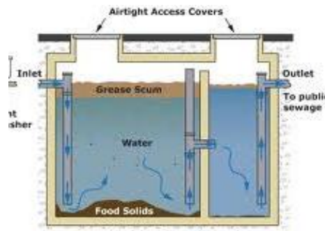
Figure 14: Schematic of Grease Trap
