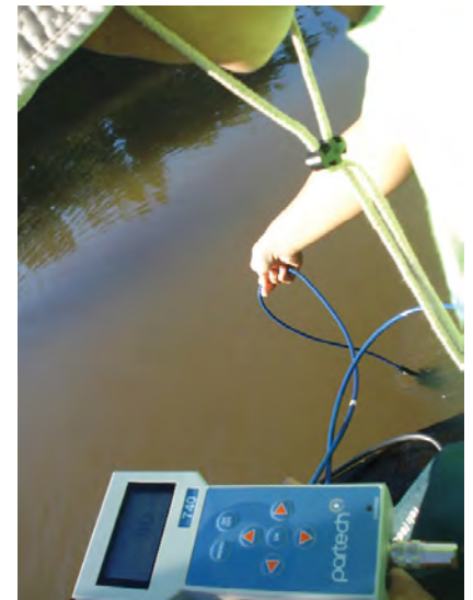
The Partech TSS Meter to monitor TSS of the Black River
